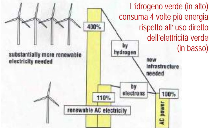
FIGURE 2. Renewable energy sources needed for electricity distribution by electrons and by hydrogen
